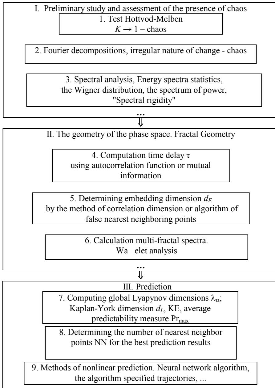
**Figure 1. Chaos and neural network-geometric approach to nonlinear analysis and forecast chaotic dynamics processes in complex systems (devices).**
