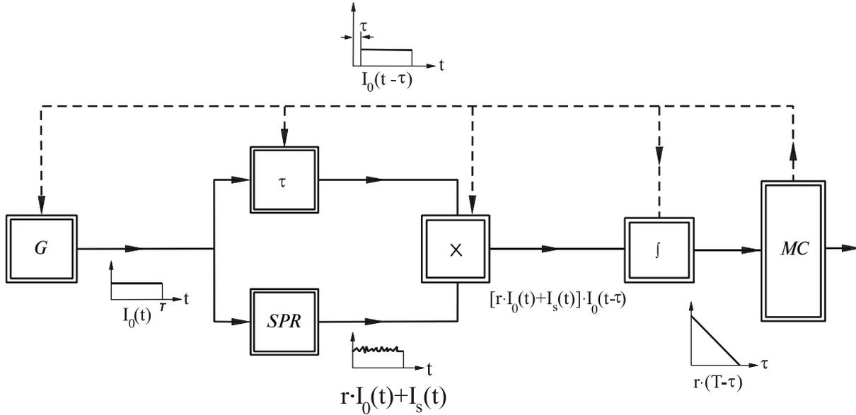
Fig.4. The functional diagram of correlation method of information processing: “G” — the generator of calibrating impulses, “SPR” — optical electronic pass of SPR-sensor, “ $\tau$ ” - the module of time delay of calibrating impulses, “ $\times$ ” — multiplication module, “ $\int$ ” — integrator, “MC” — microcomputer
