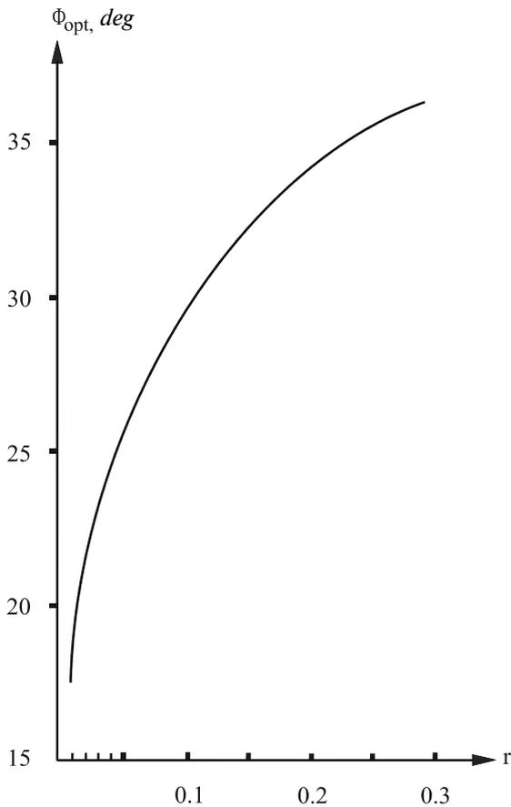
Fig.3. Correlation between  $\phi_{opt}$  and the light reflection rate  $r$  in the resonance minimum
