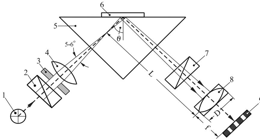
Fig. 1. The diagram of light transmission in SPR-sensor with optical phasometry: 1 — radiation source, 2 — polarizer, 3 — rectangular aperture diaphragm, 4 — cylindrical lens, 5 — total internal reflection prism, 6 — sensitive receptor, 7 — analyzer, 8 — objective lens, 9 — optical receiver
