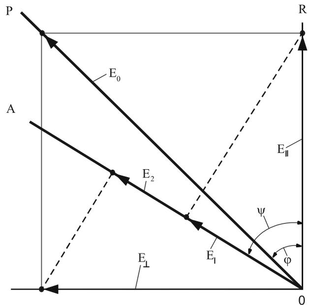
Fig.2. Vector diagram of calculating the phasometric process
