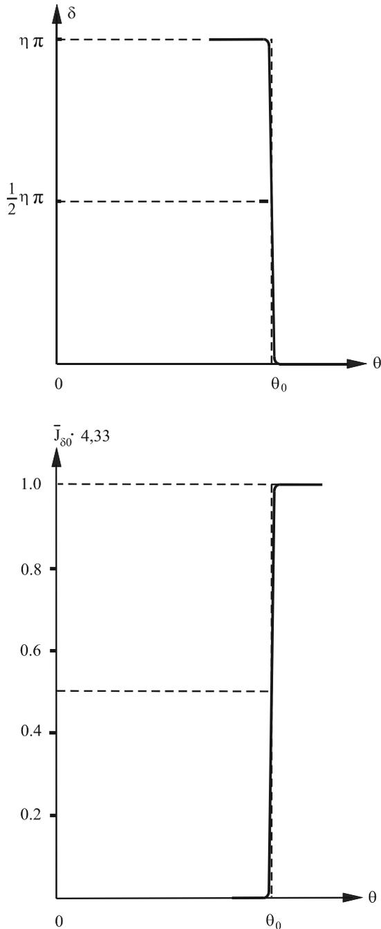
Fig.5. The dependency between phase shift  $\delta$  and correlation signal  $\bar{J}_{\delta_0}$  from angle of light incidence  $\theta$  onto sensitive receptor ( $\eta = 1, r = 0,1, \phi_{opt} = 29,35^\circ$ )
